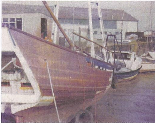
NEW PLANKING IN PLACE (the workshop in near background and caravan in front of Lochin Marine Boatbuilders)
